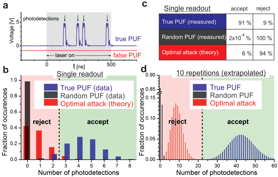
Figure 5.3: Quantum-secure readout of an unclonable physical key (PUF), using challenge pulses with 230 \pm 40 photons distributed over 1100 \pm 200 modes. (a) Real-time examples for the true key (blue line) and a false key (red line, offset for clarity). (b) Measured number of photodetections in case of the true key, a random key (imitated by sending random challenges to the same key), and for an optimal attack given S = 4 . The threshold is chosen such that the false positive and negative probabilities are approximately equally small assuming an optimal attack. (c) Acceptance and rejection probabilities in case of the true key, a random key and in case of an optimal digital emulation attack. (d) Number of photodetections extrapolated to 10 repetitions: the false positive and false negative probabilities quickly decrease to order 0.01 %.
